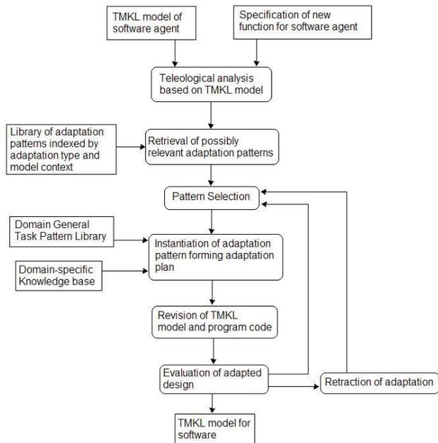
Fig. 3. REMng’s process for adaptive software design
